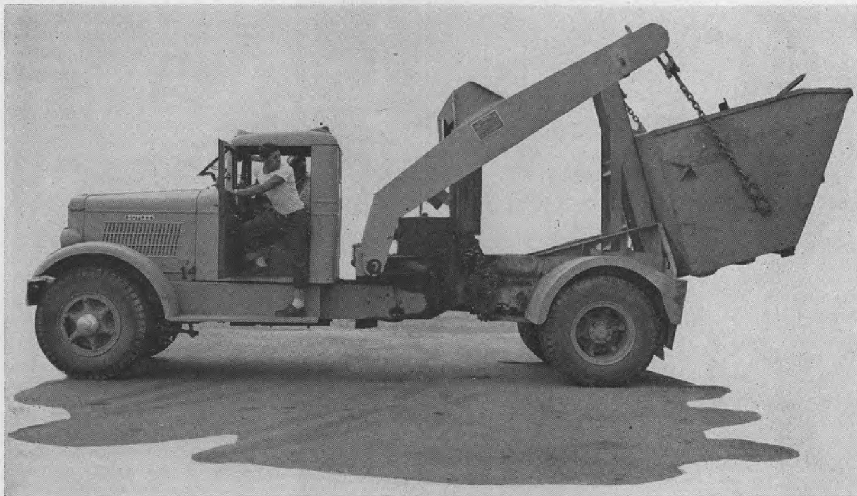
THE DEMPSTER DUMPSTER hoists one of the huge trash buckets spotted throughout the area onto its back and trundles off to dump them five miles away. Here Charlie A. Monroe, 4215, checks to see that the big bucket is being hoisted properly.
