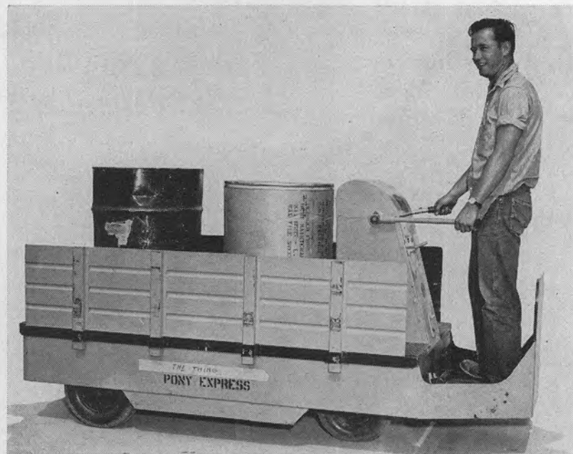
PONY EXPRESS RIDER Felix T. Miles, Jr., 2235, smiles as he drives the swift little electric carrier called the Pony Express and nicknamed The Thing. This cart is designed to transport small loads short distances fast.
