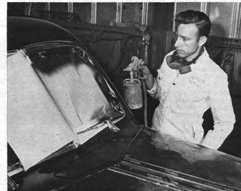
ANOTHER BUSY SPOT in the motor pool is the paint shop where Corporation cars and trucks are kept looking bright and clean. Lloyd Kelton is checking a touch-up job on a station wagon. Lloyd is an old hand at the automobile painting trade and always wears a mask while spray painting.
