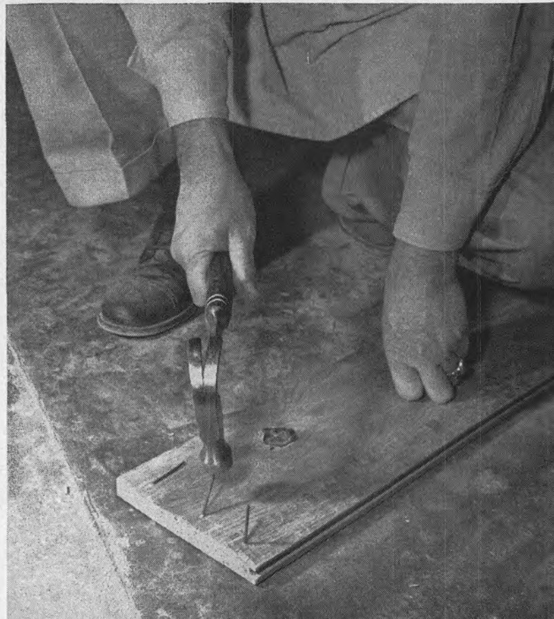
"I stepped on a nail," is a too-common statement heard from a limping or disabled householder. Be on the safe side; clinch or remove all nails on stray boards and eliminate this type of hazard.
