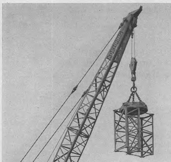
SILENT HOIST CRANE on a converted fork lift easily raises a heavily loaded copper scrap container. This crane, driven by Andres Romero, 2121, is fitted for an amazing variety of lifting and carrying operations.
