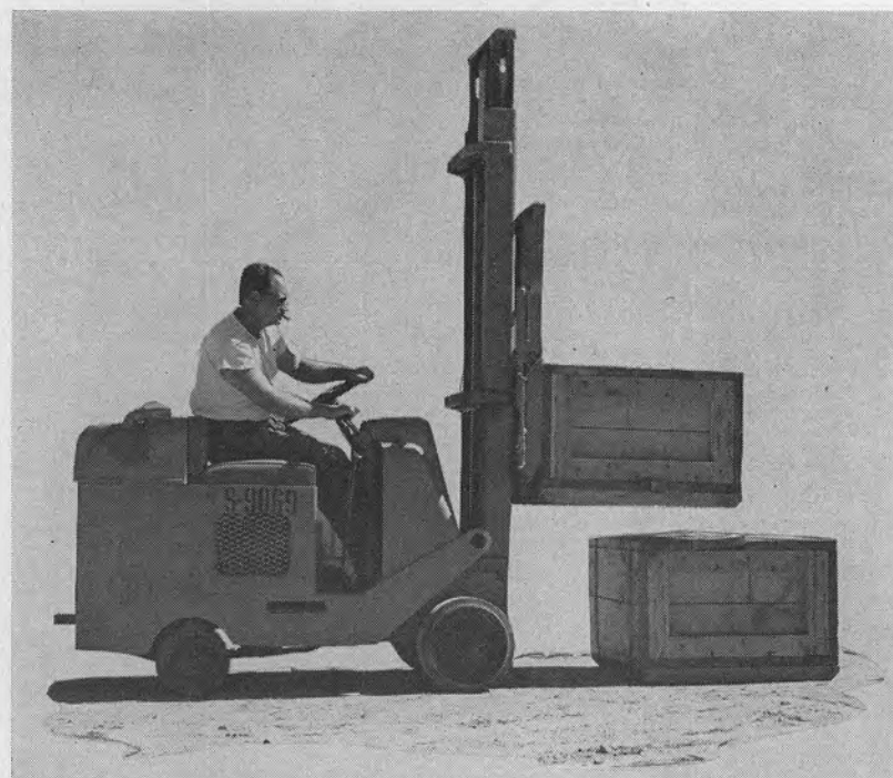
THE HANDIEST GADGET on the base is the fork lift. They come in all sizes and shapes from little box lifters to monstrous machines that can hoist 18,000 pound crates 20 feet in the air with ease. Raymond Summer, 2124-1, uses a 3,000-pound fork lift here to stack small crates.
