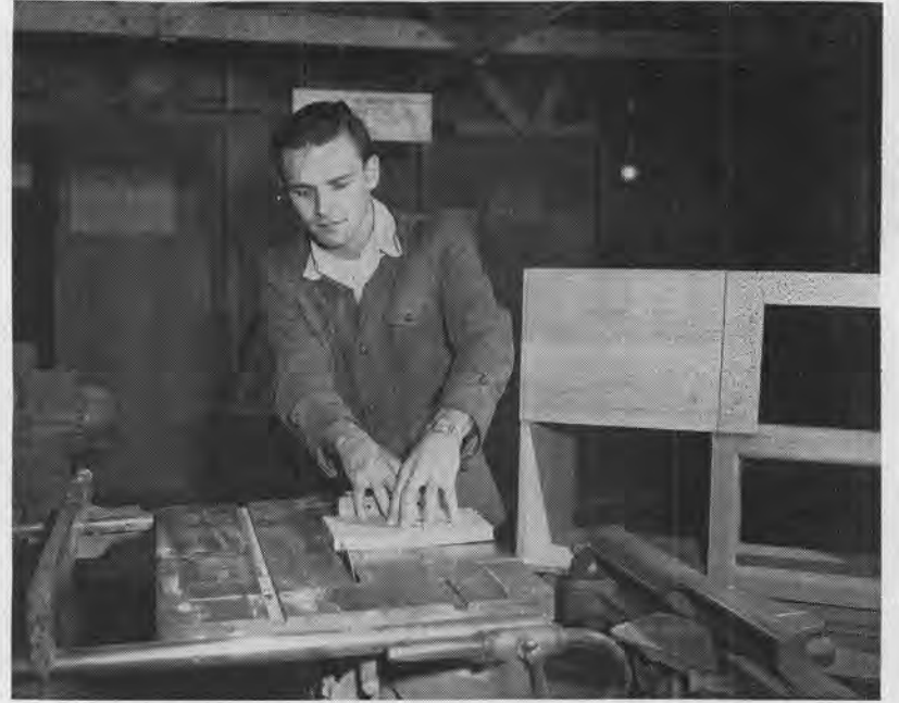
PUTTING THE FINISHING TOUCHES on a radio cabinet designed with a built-in aquarium is Kenneth Pope, 2113-4, a member of the Sandia Woodworking Hobby Shop. The saw guard was removed while the photograph was being taken. Note that Ken holds the material in such a way that his hands are not directly in line with the saw blade.
