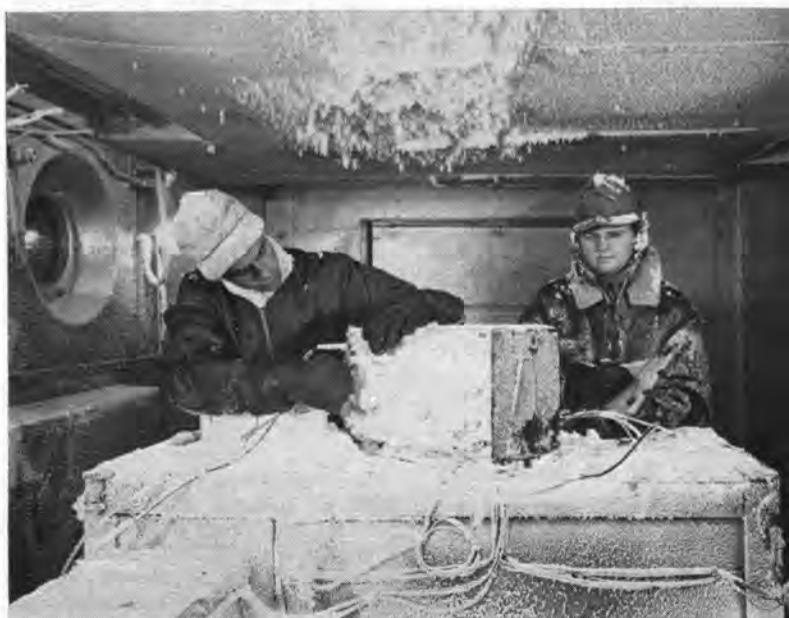
A PERFECT HOT WEATHER JOB is demonstrated by Wesley Haig, 1532, and Charles Grassham, 1531, as they check performance of equipment in 20 degree below zero weather. They don't mind this cold and frost too much. The cold chamber can be regulated to a temperature as low as minus 65 degrees Fahrenheit and sometimes they work in that frigid climate.
