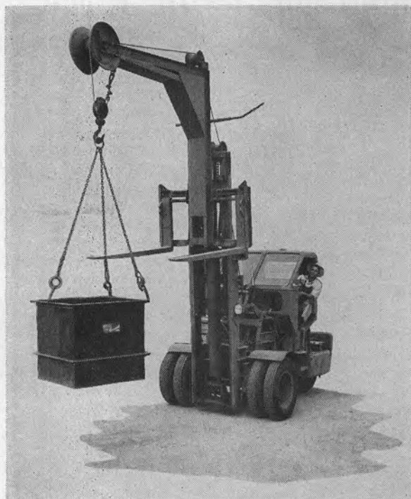
SILENT HOIST CRANE on a converted fork lift easily raises a heavily loaded copper scrap container. This crane, driven by Andres Romero, 2121, is fitted for an amazing variety of lifting and carrying operations.
