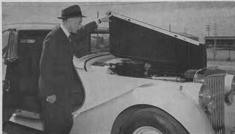
C. A. Strange lifts the hood on his new English-made Jaguar and displays the 125-horsepower six-cylinder engine. Chuck likes his cream-colored speedster, which is about the fastest car on the road.
