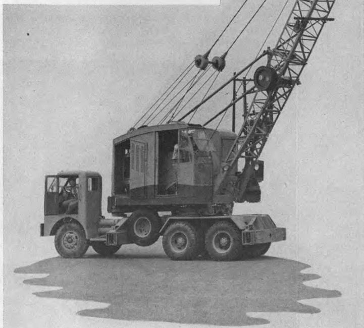
**MAGNETIC POWER LIFTS** huge crane boom sections under the watchful eye of Jesse A. Floyd, 2417, the magnetic crane operator. The big magnet can raise 5,000 pounds and when the crane is fitted with a hook it can lift 20 tons. Operating the crane tractor here is Stanley D. Brooks, 2417.
