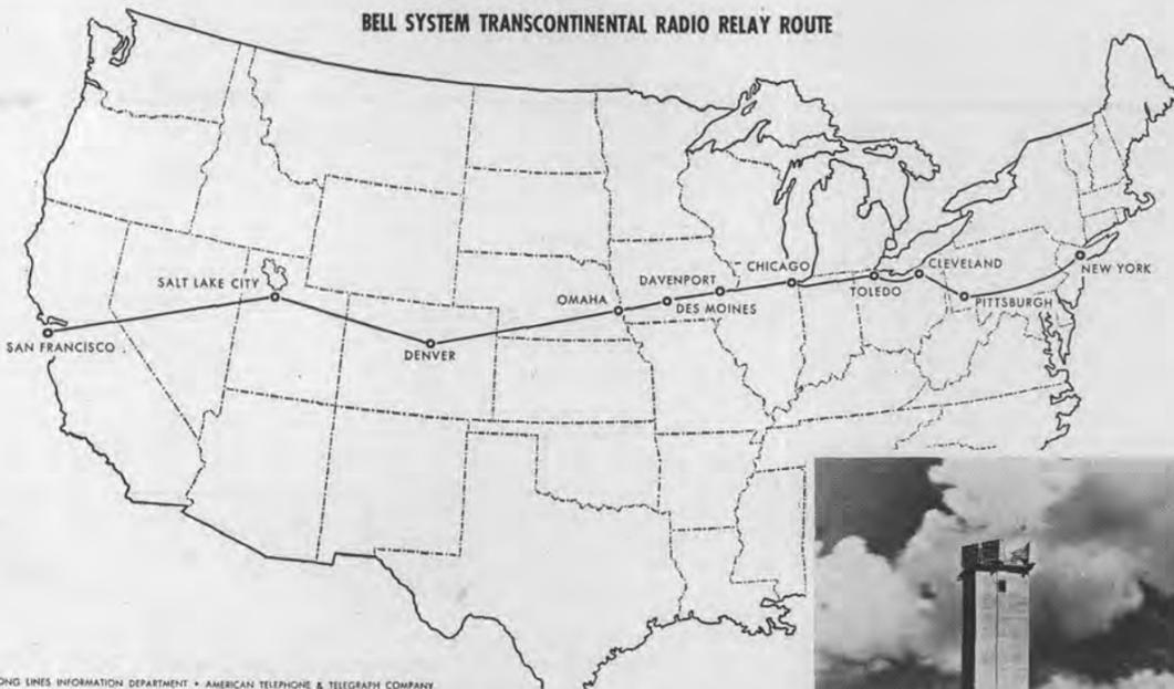
A TYPICAL CONCRETE STATION, pictured at the right, on the Long Lines Radio Relay route is located in farming country between Chicago and Des Moines. The route runs 2992 miles across the country as shown on the map above.
