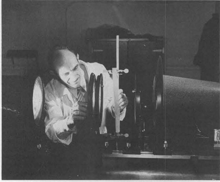
**STRESS LINES IN PLASTIC** are revealed by the polaroscope which throws a technicolor picture on a screen. Shown here adjusting the scope is Les Neeves, 1514-3. Light passing through a thick sheet of plastic set between a series of internal lenses projects a view of the plastic's internal flaws.
