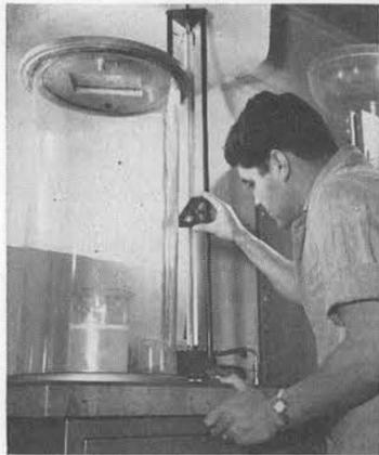
**VACUUM CHAMBER IN ACTION** produces an atmosphere pressure equivalent to 55,000 feet altitude as it sucks air out of a beaker of liquid plastic. The result is a clear plastic free from entrapped air. Lab assistant Benny Lucero, 1514-3, checks a reading on the vacuum gauge.
