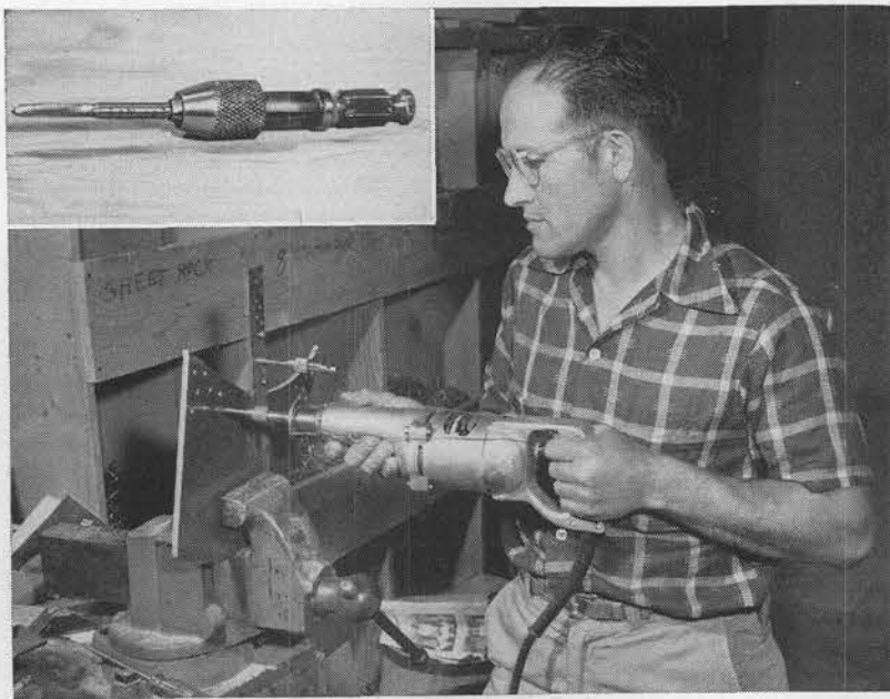
TAPPING IS EASY now that Carl Burton has designed an improvement that can be adapted to a power screw driver. The inset shows the new tapping tool he designed and the picture shows how it is used with a power machine on a heavy piece of aluminum. Screwed in the metal above it is the now old-fashioned hand tap.
