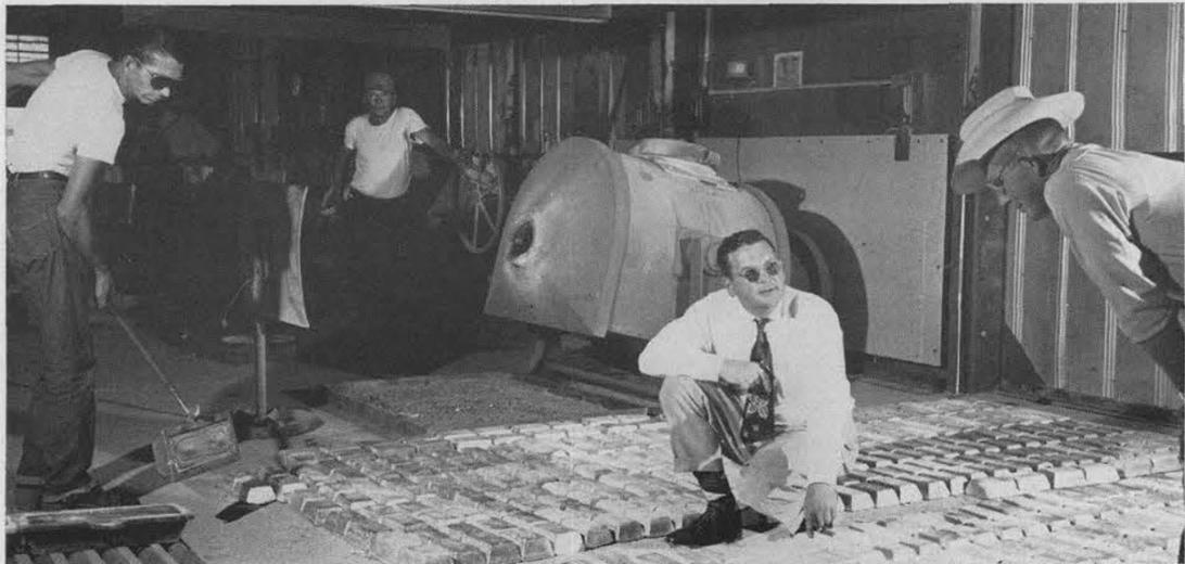
FRESH FROM THE MOLD hot aluminum ingots are laid out on the foundry floor to cool. In the center foreground **Bob Lemm**, 2352 supervisor, talks shop with **John Samuelson** while **Laddie Sladek**, left, knocks the ingots out of molds. In the background is the small tilting potless furnace used to melt down lead, tin bronze, brass and zinc. Operating this furnace is **Judson Santos**.
