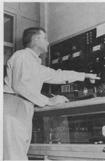
A GREAT SKILL is required to operate some of the instruments. Without it how could Harvey Skaloud calibrate a meter using the K2 potentiometer and galvanometer?
