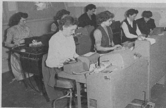
**THE STORY IS TOLD** on a card. These key punch operators have the task of operating the machine which puts the holes in detail cards. Skill and speed are necessary here.
