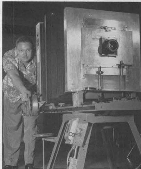
MASSIVE CAMERAS, this one operated by Elliott Harris, are used in the studios to copy technical drawings. Last year copy cameras exposed nearly 35,000 negatives.
