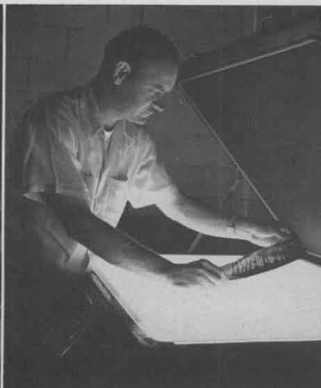
CONTACT PRINTS in sizes from an extreme miniature up to 10 feet long may be made with the printers in the darkroom. A smaller printer is operated by Kenneth Langley.
