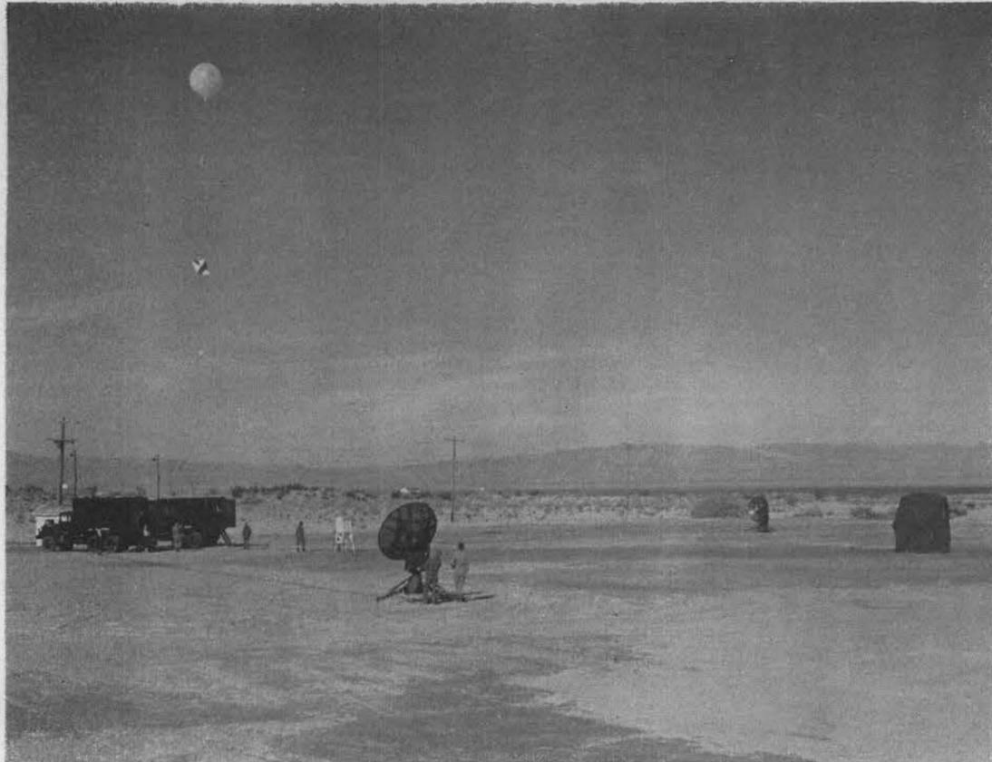
ALMOST LOST in desert wastes near Salton Sea is this mobile meteorological unit, shown making radiosonde observations on winds and air currents aloft. Balloon carries radar kite, radiosonde transmitter which emits information as to speed of winds, direction, to receiving instruments on the ground.
