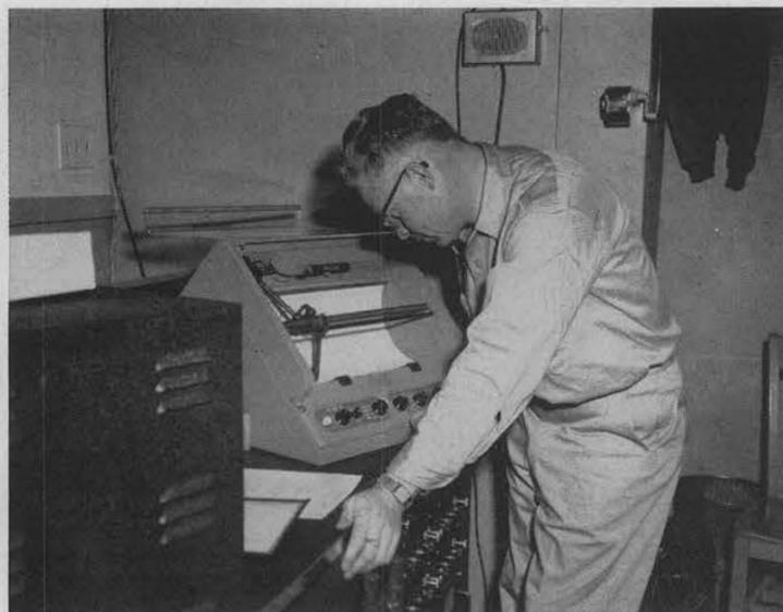
**RAYPAC COMPUTER**—Everett F. Cox, 5110, prepared the "mechanical mind" (more accurately the ray path computer) before the first shot of Operation Teapot.
