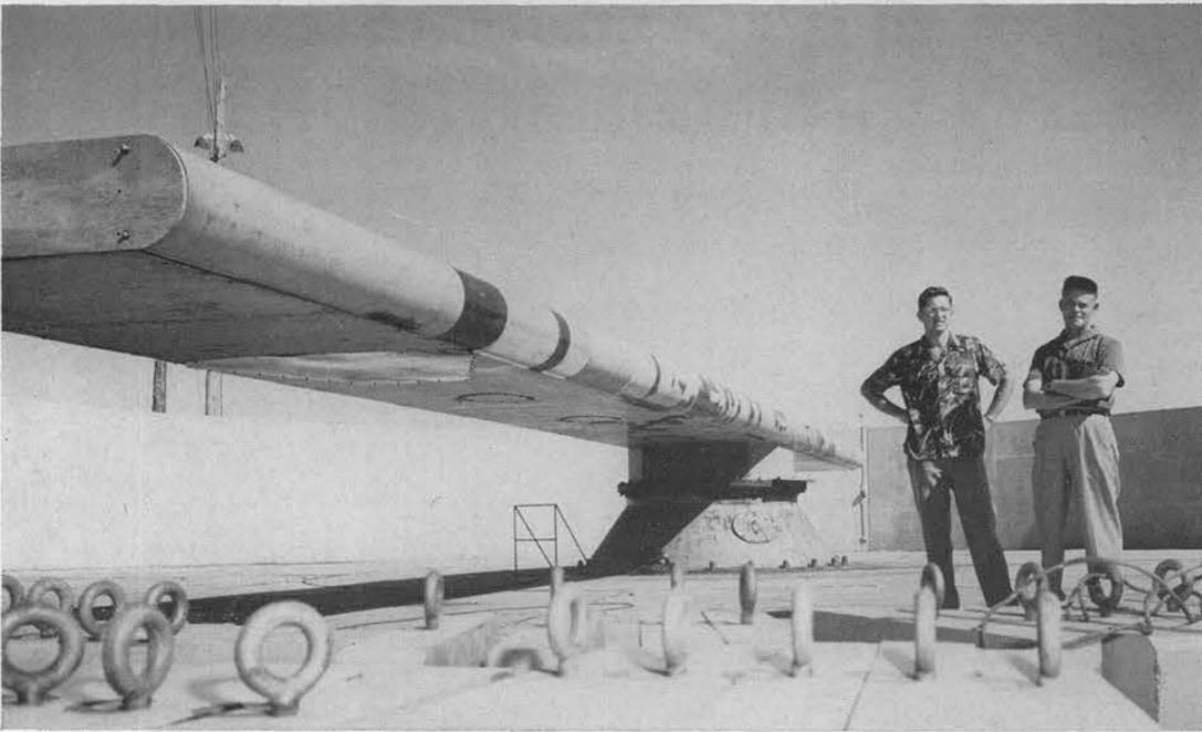
**HUGE STEEL BOOM** of the hydraulic centrifuge dwarfs its operators, Milton Jones, left and Don McCoy. In the foreground are rows of heavy steel weights used as counterbalances during Tech Area centrifuge tests.
