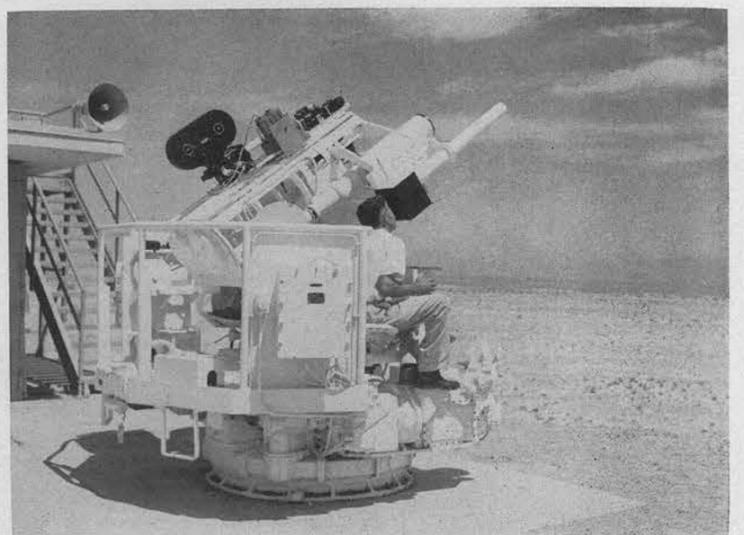
EYES of movie camera are focused on falling bomb by operator of automatic tracking device mounted on former anti-aircraft gun chassis.
