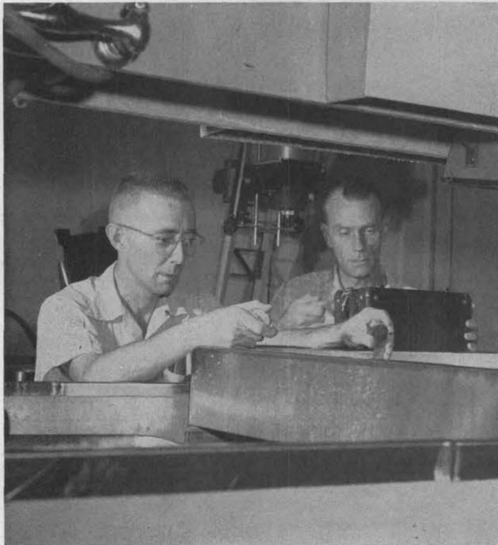
INDUSTRIAL HYGIENE technicians, Garvey Pierson, left, and Allen Hobbs, monitor "hypos" trays in Sandia Corporation photographic laboratories, testing content of "hypos" in air.
