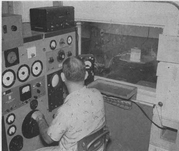
VIBRATION MISERIES — The howl of a shake table, seen through the window of a soundproof room, would greatly irritate operators if it were not safely enclosed as shown here. This is but one example of how the industrial hygienist makes working conditions more pleasant.
