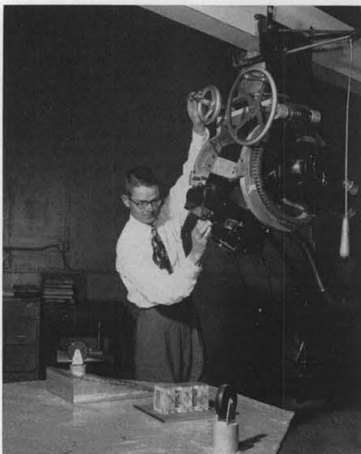
INDUSTRIAL X-RAY INSPECTION is made of electronic unit by Osborne Milton, 1612, in a search for hidden flaws. X-Ray can be used to detect cracks and distortions unseen by naked eye, is also employed in analyzing crystalline materials. In the Test Laboratory Department, X-Ray Inspection equipment includes Diffraction X-Rays, 250 KV X-Ray machines, and an AEC Gamma Ray source with great penetrating ability.
