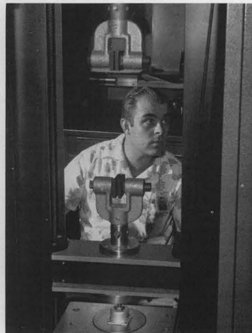
PROOF TESTING of components is performed by Richard Bohannon, 1611, who operates device to "squeeze" small aluminum container with predetermined pressures. Tests like these give scientists an idea of effects of stress and strain on various weapons parts.
