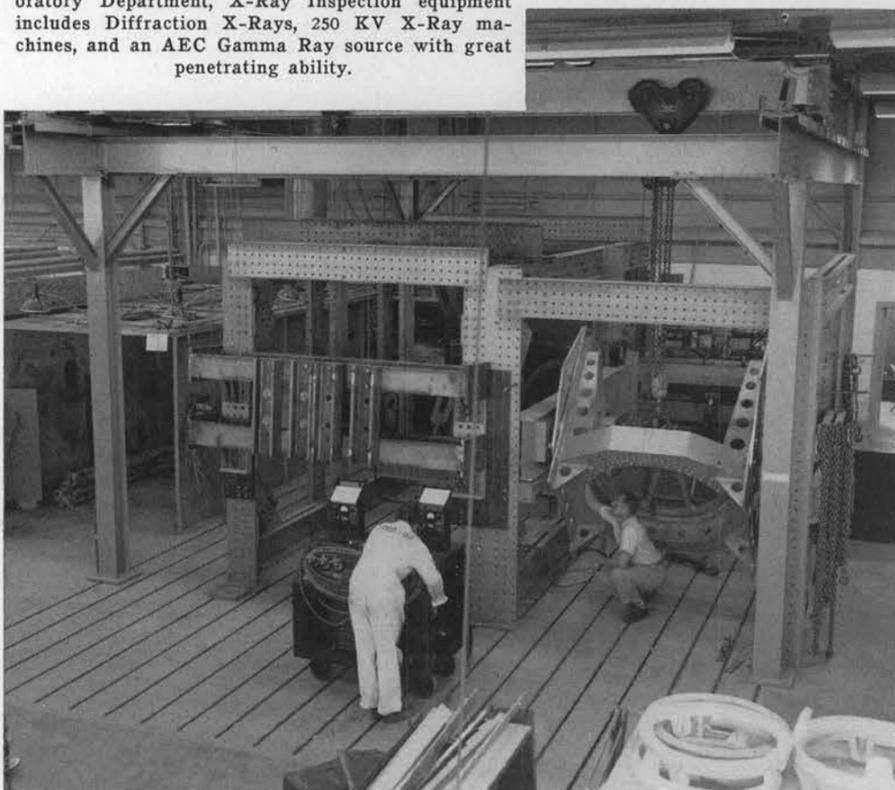
BIG STATIC JIG helps provide fundamental data on stress-strain problems. This roomful of steel girders in Bldg. 860 is used to test assemblies up to 25 feet long, is an important tool in evaluating mechanical properties of units. Adjusting control console, left, is Andy Imrisek, and right, Elmer White, both of 1612-2.
