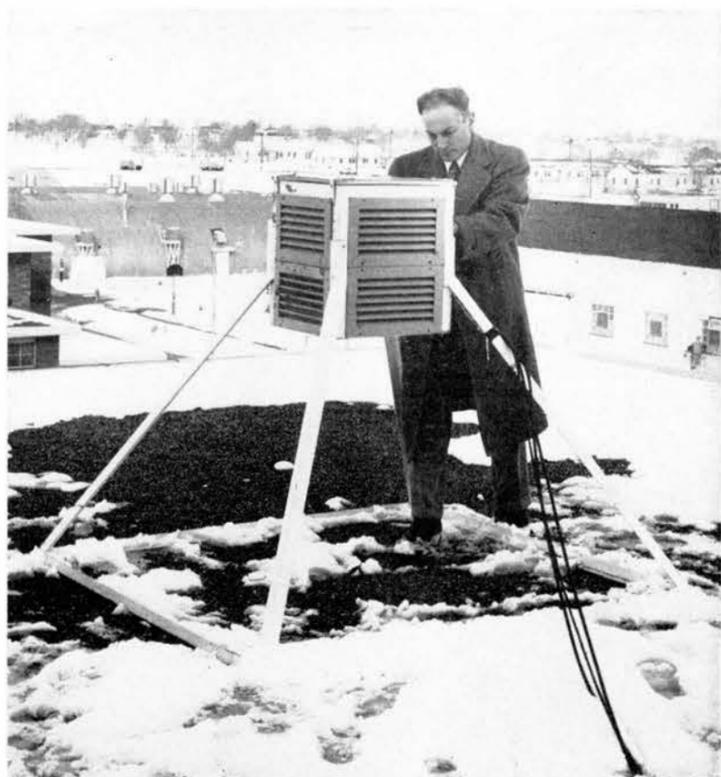
MEASURES RADIATION—Howard H. Sander, a Sandia Corporation engineer in the Weapons Effects Department, 5110, stands beside the instrument which helped measure radiation fallout from the 1955 test series in Nevada. The device showed that the total dose increase of background radiation in Albuquerque amounted to about the same one would receive by wearing a radium dial wrist watch for a year.
