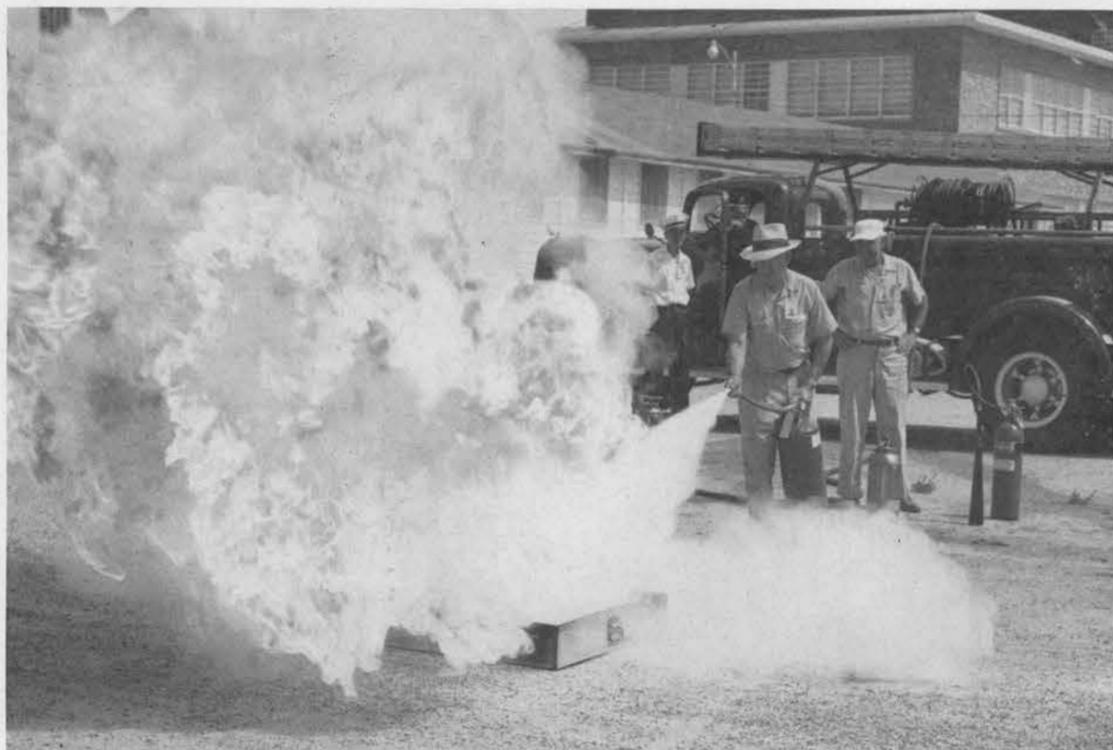
DEMONSTRATION of fire extinguisher types and methods of using them is conducted during the year by Plant Inspection Division, 2442. Here Ted Rosenwald uses a dry chemical extinguisher on a flammable liquid fire as a Base Fire Department truck stands by to be used in a later demonstration.
