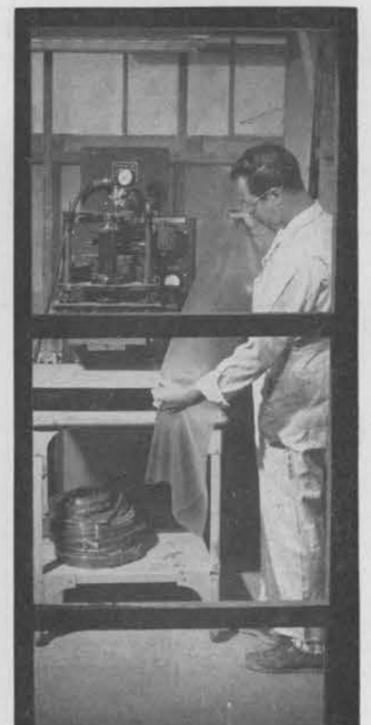
MICROWAVE PRESS welds seams in vinyl film. Kenneth L. Peterson operates the machine which generates heat through molecular action in material.
