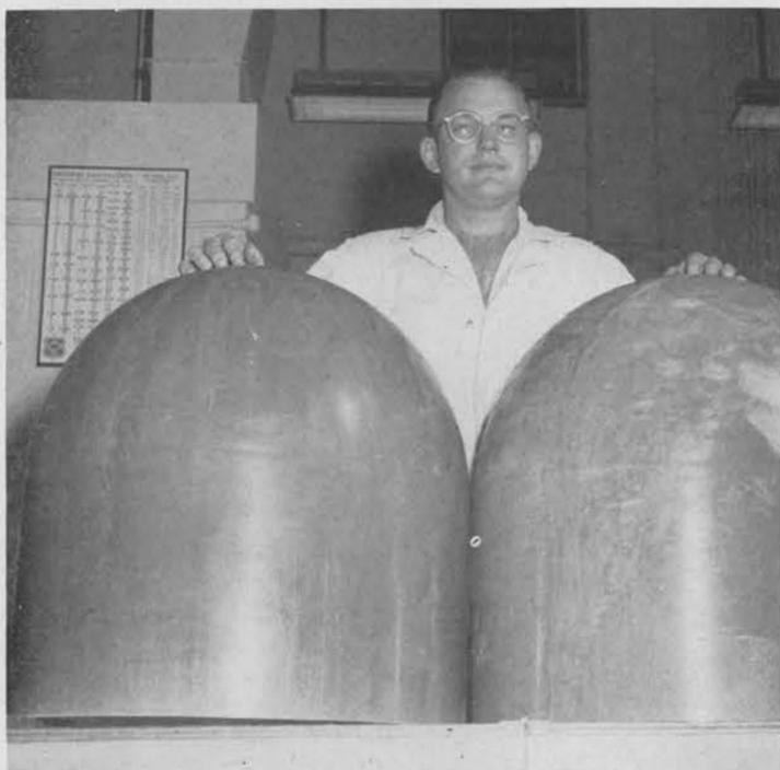
FINISHED DUST COVERS are shown by Richard Olive. After the glass cloth and resin lay-up is completed, the entire mold is covered with a plastic bag and a vacuum created to force the air out.
