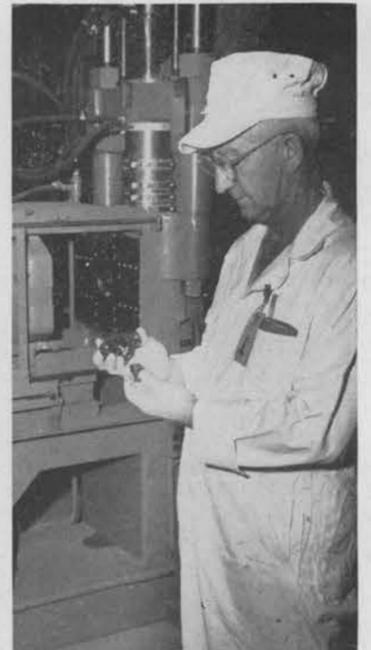
INJECTION MOLDING machine operated by Marvin Harvey is capable of producing small precision pieces in great quantities. A hopper feeds dry plastic powder into the machine's heating chamber where it is melted into a thick liquid. This liquid is forced into the mold where it is formed and chilled almost simultaneously.
