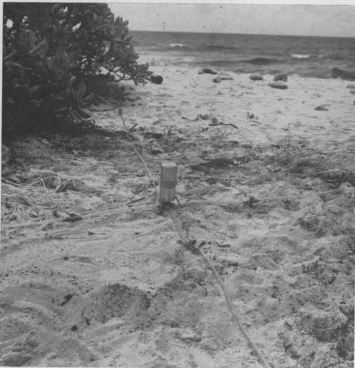
MICROBAROGRAPH "head" site on a lonely stretch of Ronjerik beach. Plastic tubes and fittings filter out the sound of the surf.
