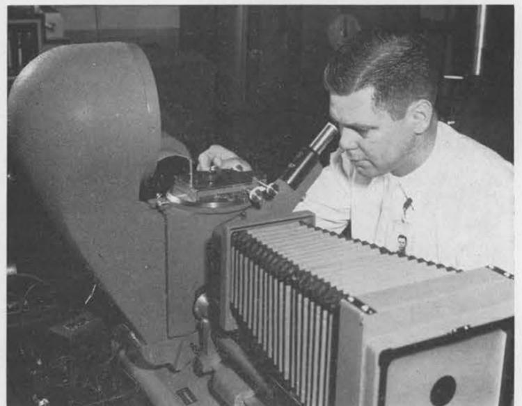
**MICRO-STRUCTURE** of a metal specimen is studied by Keith E. Mead, Supervisor of the Metallurgical Section of the Materials Laboratory Division, 1621. The instrument used is a Balphot Metallograph which enables the operator to see crystal structure, impurities, inclusions and distribution of ingredients in the specimen. The Metallograph includes a camera to make photographic records.
