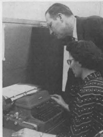
READYING COPY for reproduction, using a tape-operated typewriter, is Mildred Hinds. Art Lites, supervisor of the Composition Section, 7121-1, observes operation of the machine.
