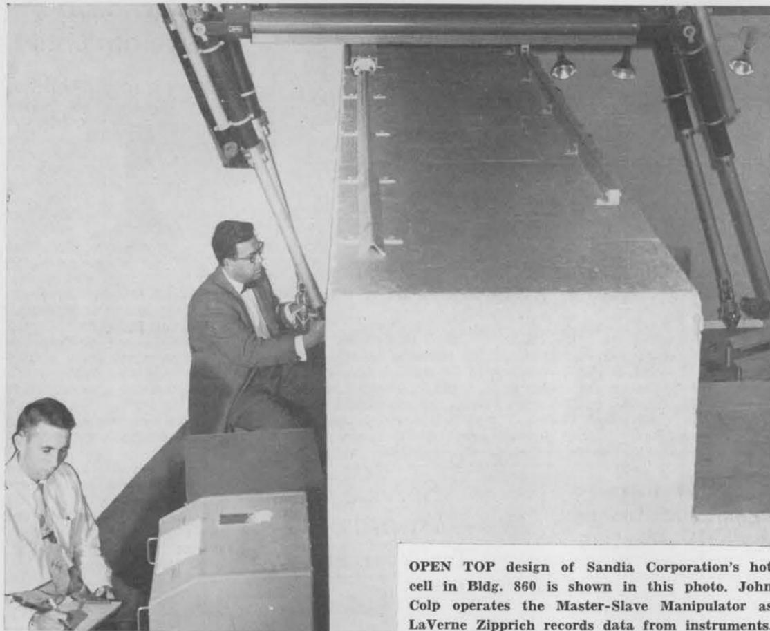
OPEN TOP design of Sandia Corporation's hot cell in Bldg. 860 is shown in this photo. John Colp operates the Master-Slave Manipulator as LaVerne Zipprich records data from instruments.
