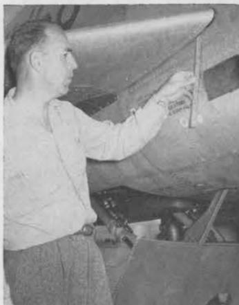
BURTON S. SNOW inspects a camera window opening on a modified U. S. Air Force F 100D.
