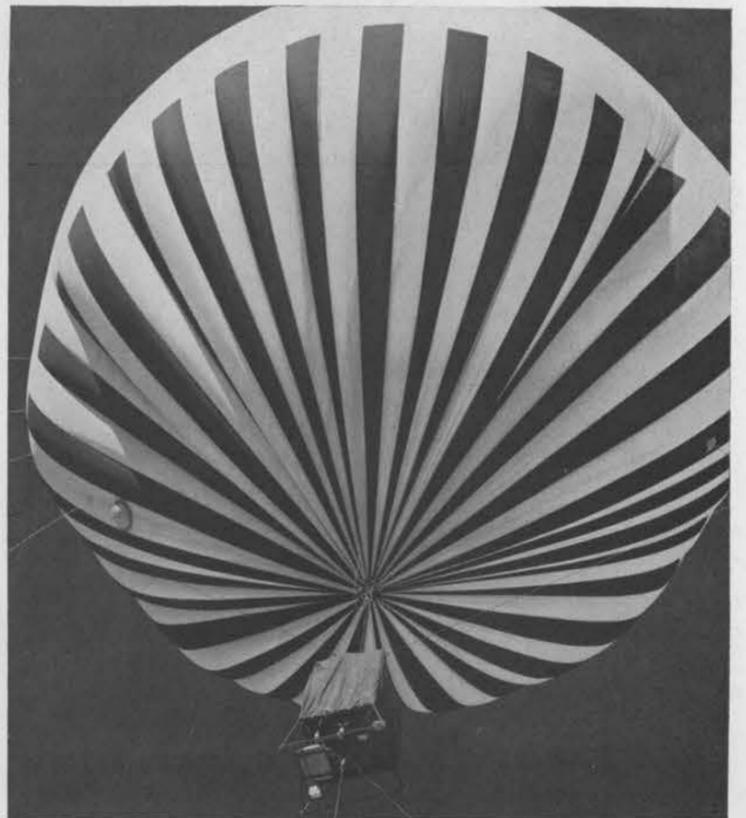
**INFLATION** is accomplished by inserting a metal probe with thousands of holes into a plastic filler tube attached at the bottom of the big balloon.
