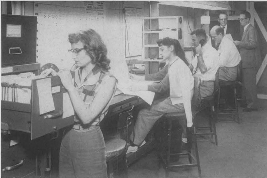
**VISUAL INSPECTION** for missing cables, labels and nomenclature is performed at Santa Barbara Electrical Products while field representative Ray Lewis, right, watches. Inspection for electrical and mechanical performance will follow this check. Ray is a Sandian from the Los Angeles Office.
