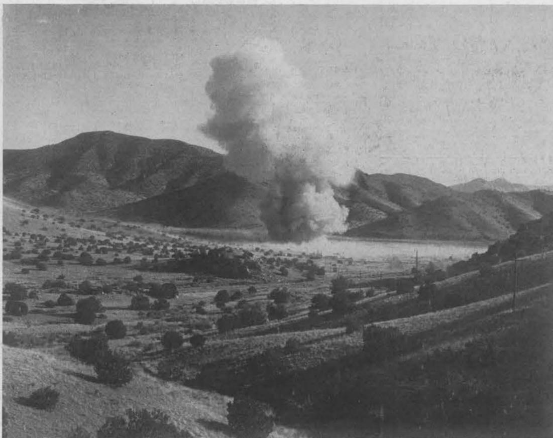
**SCALED BLAST** at Coyote Canyon almost duplicates the mushroom cloud of a nuclear explosion. This shot was six tons of TNT, the largest ever exploded at Coyote Canyon, and duplicated in scale the effects of a 20 kiloton atomic explosion. Blast diffraction studies continue in the Canyon.
