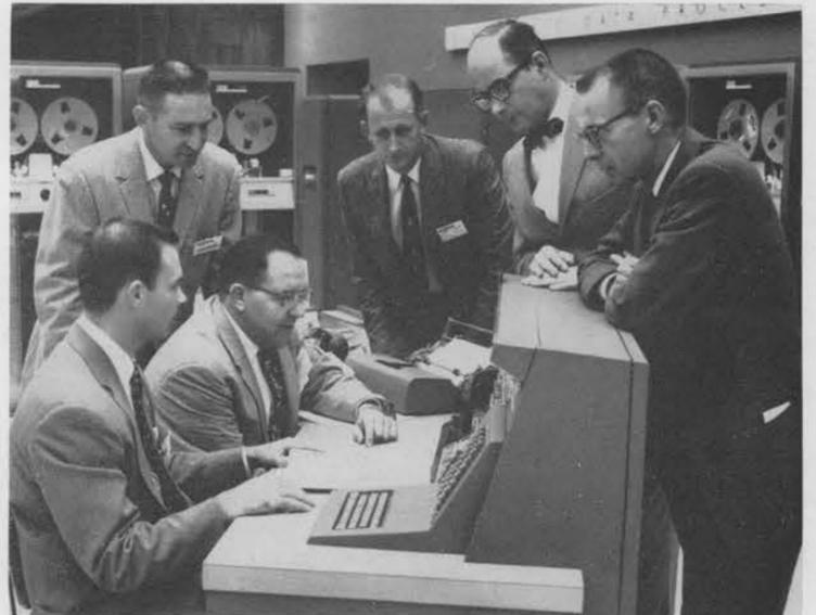
CONTROL CONSOLE of the 705 is studied by Sandia EDPM specialists. The console permits the operator to supervise 705 functions.
