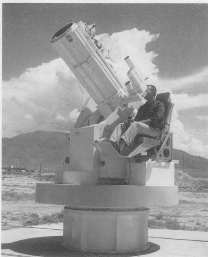
AN EYE WITH A BRAIN is this newest Sandia tracking telescope now in operation at Tonopah. The instrument, shown going through shake-down tests in Albuquerque, is operated here by Joel Hamilton (5224). The control stick in his hand activates an "electronic memory" which tracks objects almost automatically.
