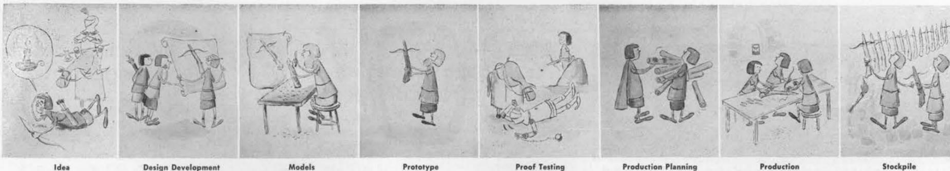
Idea Design Development Models Prototype Proof Testing Production Planning Production Stockpile
