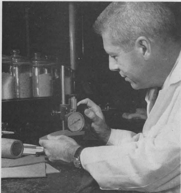
**TESTING HARDNESS** of rubber is George Dykes (1625). This is one of the many tests new materials must undergo in the development of experimental weapon components at Sandia Corporation.
