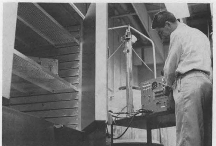
HOT CHAMBER to simulate extreme conditions is used by James R. Collier (5522). Quality evaluation runs the gamut of temperature extremes, humidity and vibration to check parts performances.
