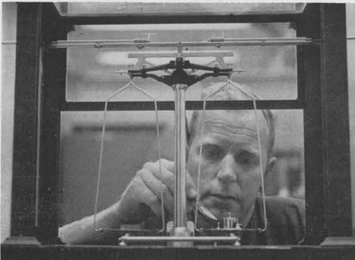
STANDARDS for nuclear weapon parts are exact; some kinds of discrepancies cannot be tolerated. Here George Johnson (5531-3) uses analytical balance scales to check an engineering requirement.
