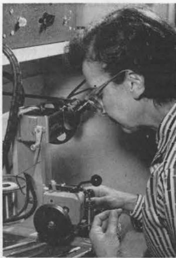
**MECHANICAL WINDER, operated by Lois Donaghy (2133), has already placed 900 turns of No. 50 wire onto a core. Six wires are attached and numbered.**
