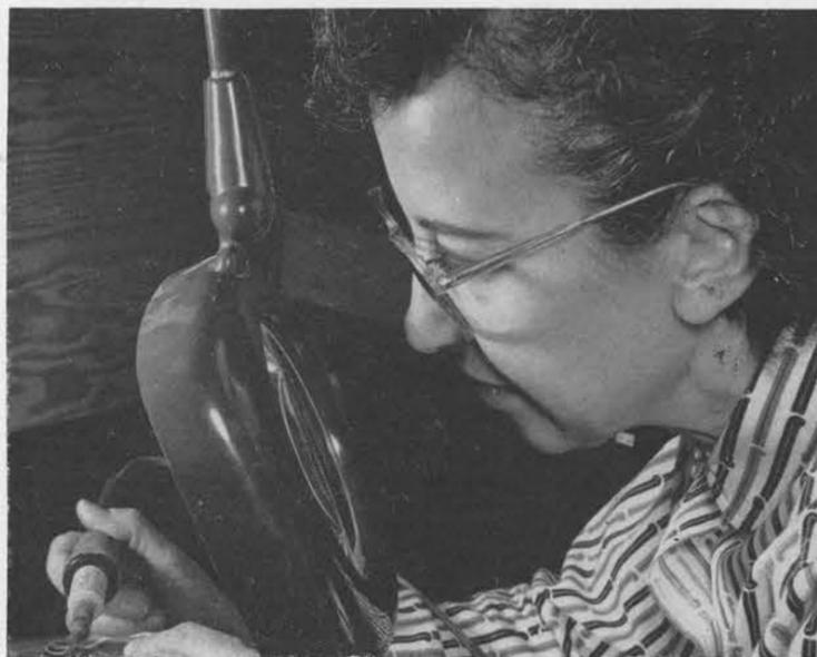
**WOUND COIL is mounted on heavy assembly jig for ease in soldering lead out wires onto terminals. A resin coating is added later.**
