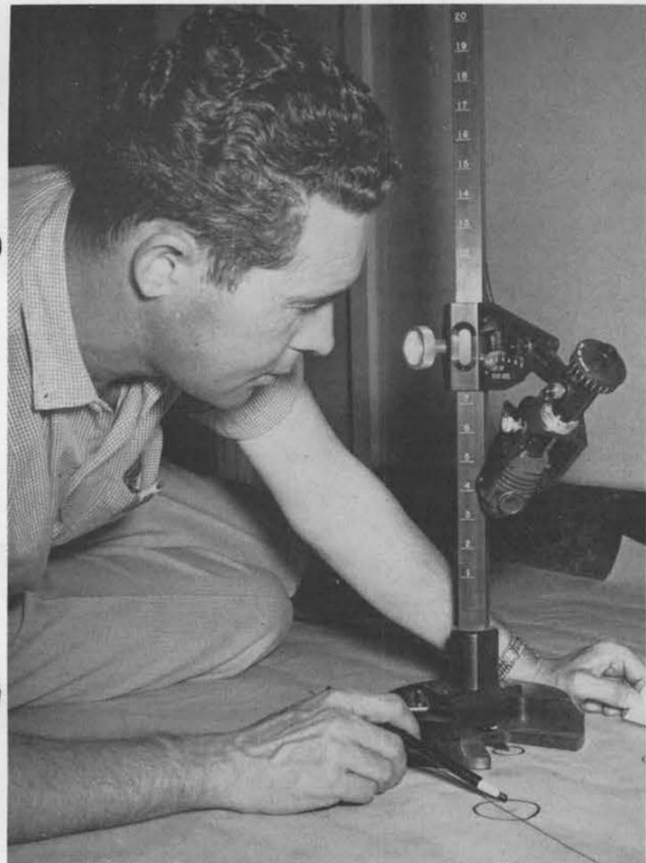
TAKING A READING on Sandia's solar computer is J. M. Allen of the Flight Test Division (5211). The computer is used to plan the times of test operations at Sandia's ballistic ranges, assuring that the sun won't interfere during filming of test drops.
