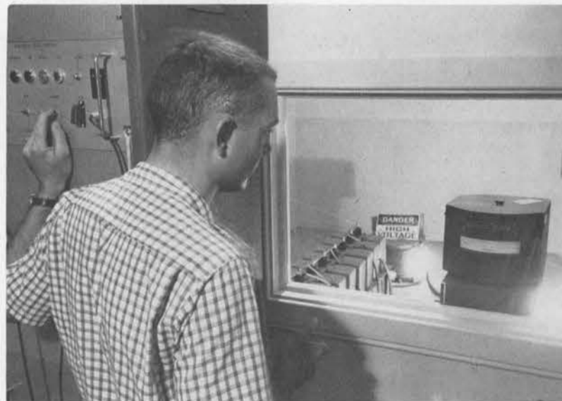
HIGH VOLTAGE is fired through a dummy load in connection with "Sherwood" engineering studies being performed by the Special Projects Division (1265). Allen Church throws a switch and a shorting wire on the load is completely vaporized.
