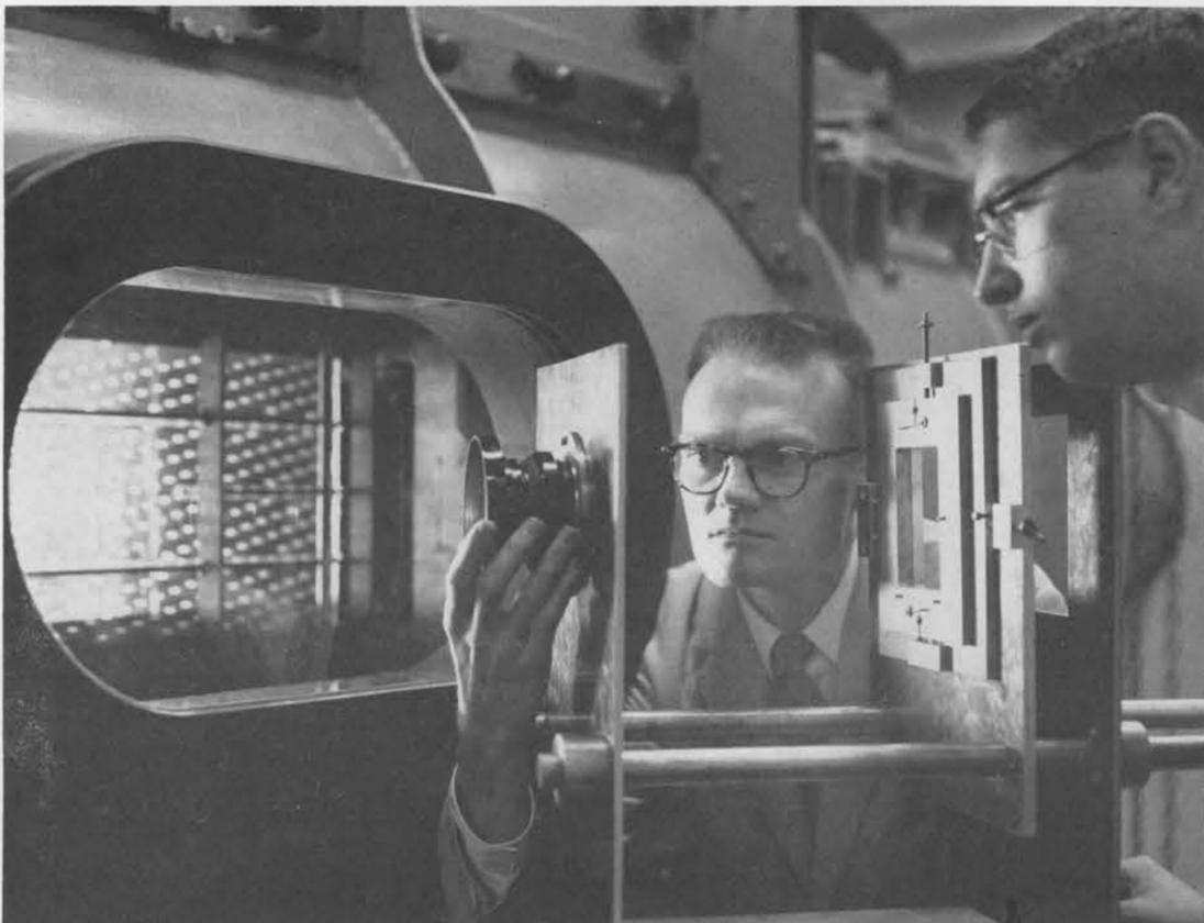
SHOCK WAVE PHOTOS in Sandia Wind Tunnel were made possible with this camera, which is being assembled by its designer R. E. Krylach (5224), left. Looking on is Harold Spahr, Jr., (5142).
