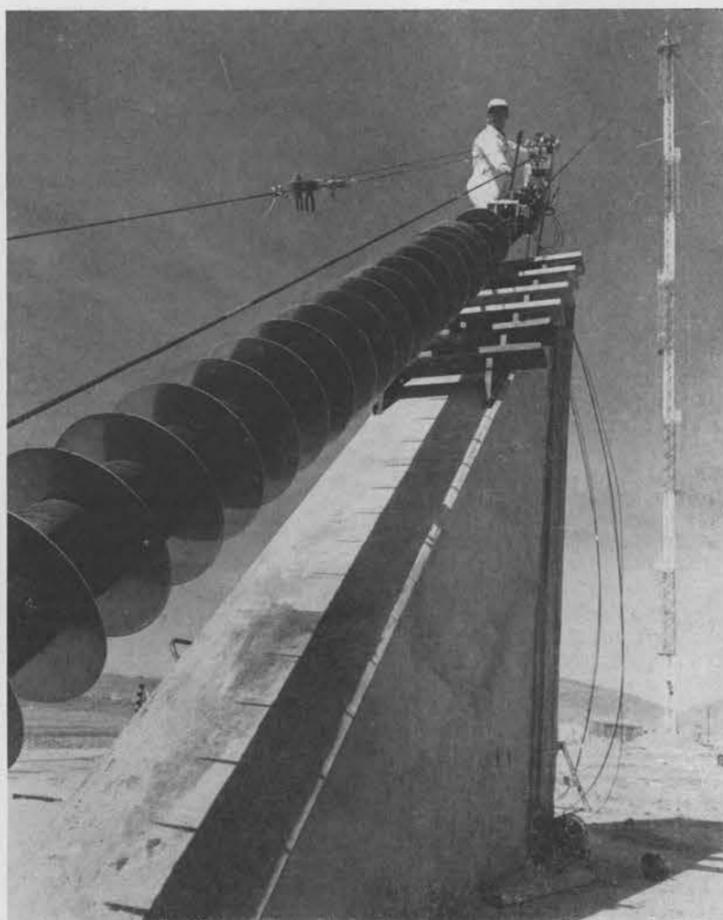
SHOCK ABSORBERS on 300-foot drop tower in Area III check recoil when cart descends cable. The tower is used to test the effects of shock on a variety of strategic materials.
