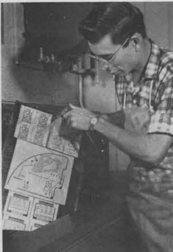
DEVELOPING the image on the laminate is performed by Kenny Anderson. Here he washes excess dye from the plate leaving only the exposed writing pattern visible on the copper.
