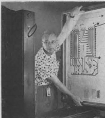
MASTER NEGATIVE is produced in this huge copy camera by Leonard Malkowski. The duplicate master about to be photographed here will be reduced about four to one in size on the copy camera's negative.
