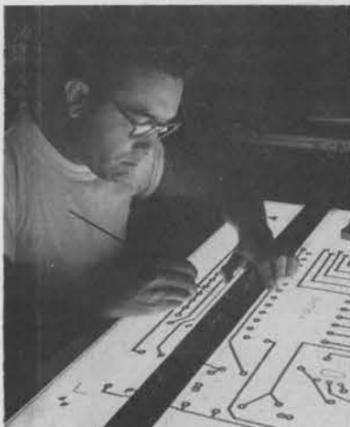
TOUCHING UP a duplicate master, a contact photographic print of the original drawing, is done by Bob Velasquez. He checks for defects and adds any necessary markings for the production of the circuits.
