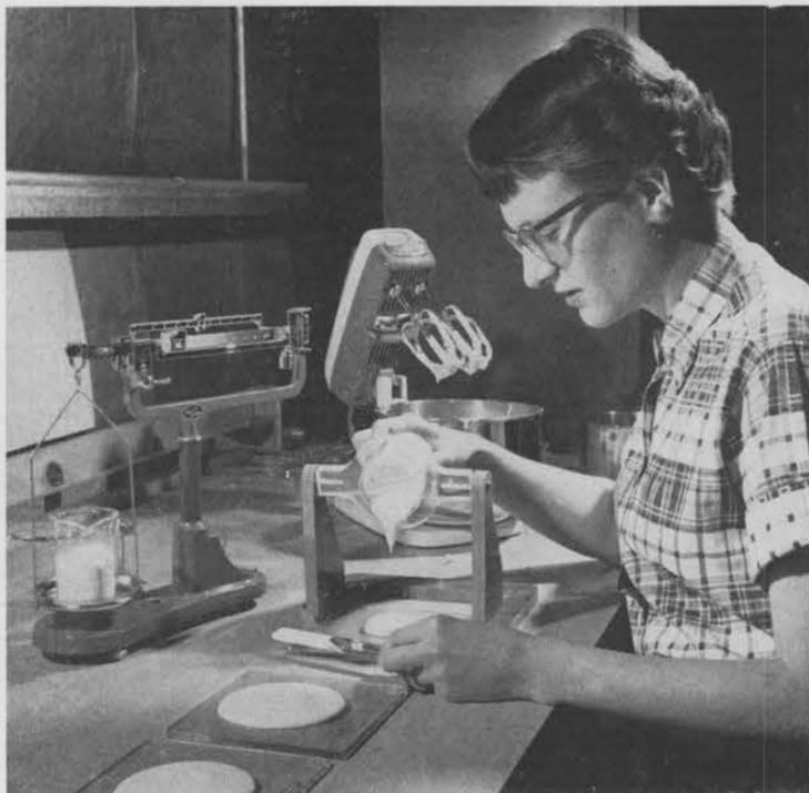
**STRENGTH AND CHARACTERISTICS** of the materials in which the miniature craters are exploded are carefully plotted by Nancy Feight, above. She is shown mixing the samples which will be used as a guide when actually pouring the blasting blocks.
