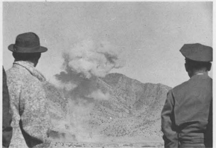
**TOPPING OUT**, the cloud towers over the Manzanos, but there will be no "fallout" because it is a non-nuclear test, set off in Sandia's Backyard Bikini to provide information to be used in planning peaceful applications of nuclear blasts, such as mining and harbor work. The work is performed under the direction of D. G. Palmer (5112), with cooperation of many Sandia groups.
