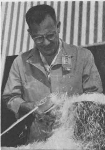
**LIKE CAKE FROSTING,** glass fibers spray from a hand-held chopper to a plastic-coated part. Alternating layers of fiberglass and plastic spray produce a strong fiberglass laminate. The chopper being used by Don Beard (8115-2) was developed by 8115 for this type operation.
