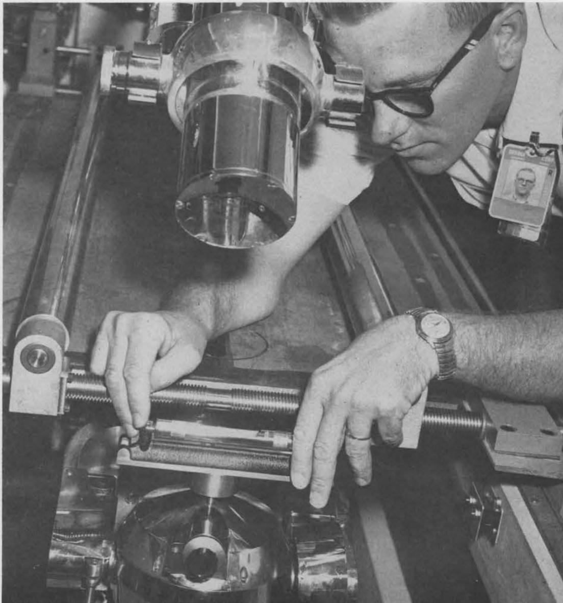
**ADJUSTING** the radiation source holder on the DXT Machine is Harry Olson (8115-1). DXT means **Density Times Thickness.** The machine uses radiation to precisely measure materials density variation.
