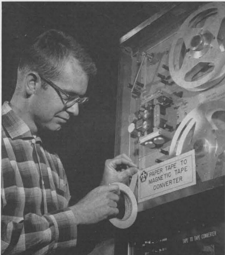
**UNIFORM SIGNS** bearing official thunderbird design will be used throughout Tech Area I during Family Day to identify equipment or facilities. Kenneth A. Bixler (5243-4) fastens lettered sign onto Automated Data System, developed by Sandia's organization 1500. The complex machine converts punched paper tape to magnetic tape for use in the IBM 704 or 705. Display is in room 36 of Bldg. 880.
