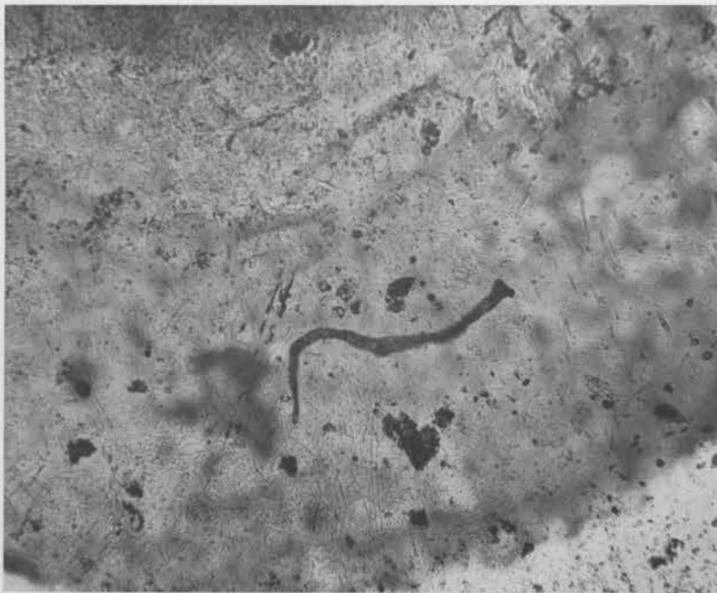
**MICROSCOPIC DEBRIS** on an electrical contact looks like this when magnified 108 times. The snake-like object in the center is a minute nylon fiber about 1/50th of an inch long. Other spots are metallic dust and foreign materials. Microchemists of 1621-3 detect and identify the debris and find means of avoiding it in the production of electrical contacts necessary for various components.
