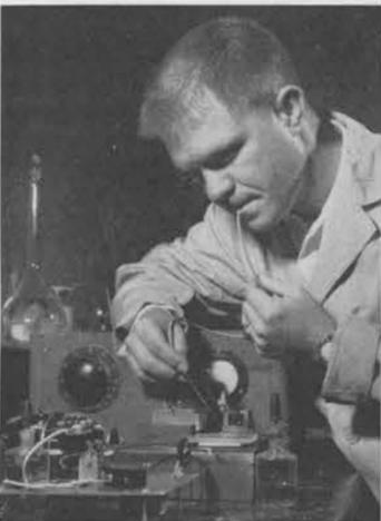
**CHEMICAL TEST** on an electrical contact is performed by Don Fjelseth. He is placing a very small drop of sodium oxide on the contact surface which will react if sulphide is present.
