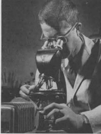
**BASIC TOOL** of the Microchemistry Laboratory is the microscope. Here Lew Jones studies a plastic replica specimen from a contact to optically analyze foreign matter on its surfaces. Area under observation is somewhat smaller than this period.
