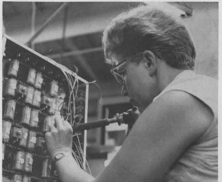
**CAREFULLY SOLDERING** connection in an automatic production tester is Dorcas Richie (2551-3). After fabrication the production tester of nuclear components is "proved-in" by section 2551-4.
