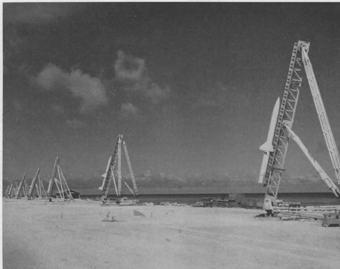
SANDIA HIGH ALTITUDE research rockets stand poised to roar into fireballs of ORANGE and TEAK shots. The large two-stage rockets carried instruments for making measurements of nuclear radia-
