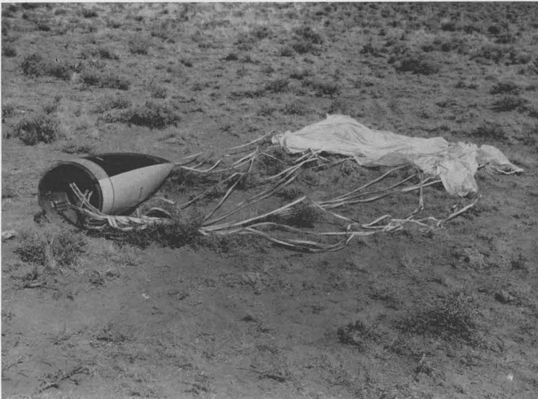
RECOVERABLE NOSE CONE of Sandia's high altitude research rockets is shown in photograph above. The parachute mechanism floats nose cone to the ground and allows for recovery of delicate payload of instruments and recorded data. The nose section is recoverable from land or water.
