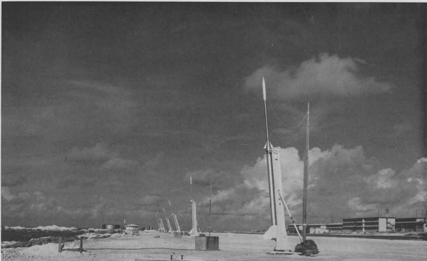
SMALL TWO STAGE ROCKETS developed by Sandia were used for RF attenuation studies of ORANGE and TEAK shots. Some of these rockets carried chaff ejecting heads for high altitude wind measur-
