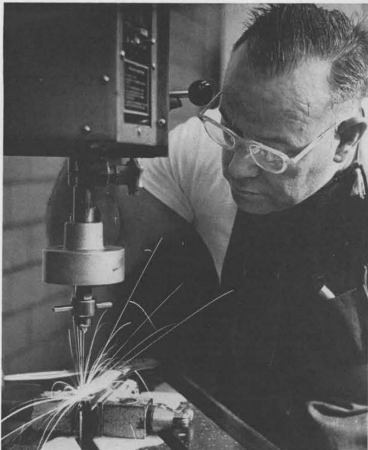
**SPARKS FLY** as John Moffet uses an electron drill to center drill a cylinder of alnico. The machine progresses at the rate of  $\frac{1}{2}$  inch every 11 minutes and is an extremely accurate machine tool.
