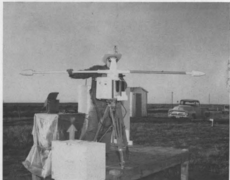
FLIGHT ANALYZER camera is operated by V. E. Baker (5216) during test drop at Dalhart Range. Some cameras are automated.
