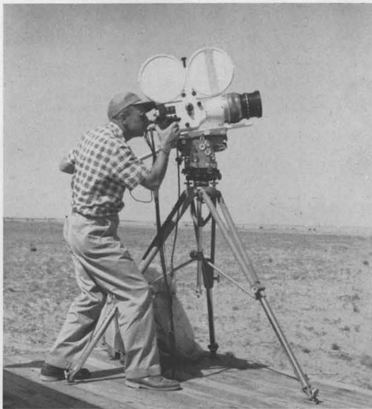
HIGH SPEED 35mm movie camera, operated by N. L. Richardson (5216), provides additional data for study. This camera can take 1500 frames per second. Normal projection speed slows action.
