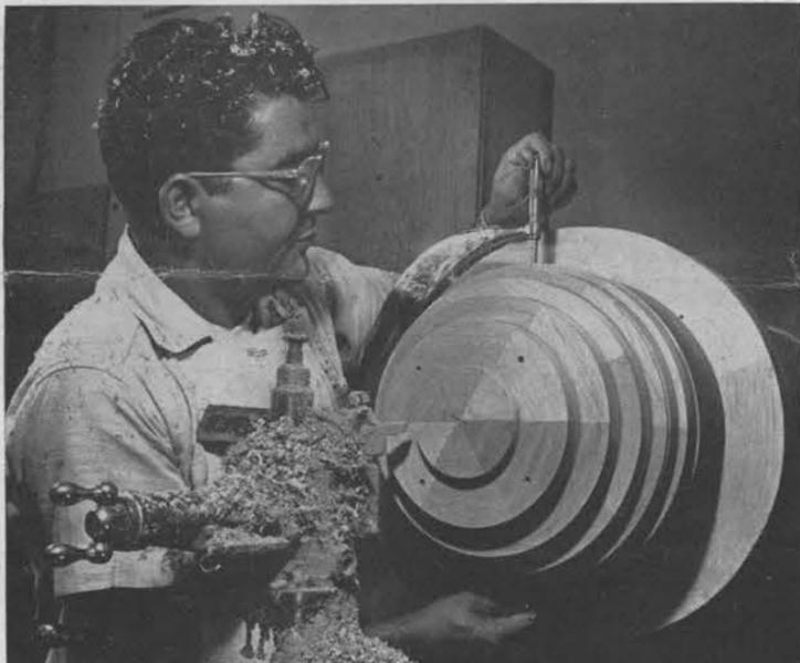
**ESTABLISHING CONTOUR** stations in a laminated pattern prior to machining is J. J. Atencio. He is precision measuring the piece with a micrometer. Contour forming is mainly a hand operation using a template for continuous checking of accuracy.
