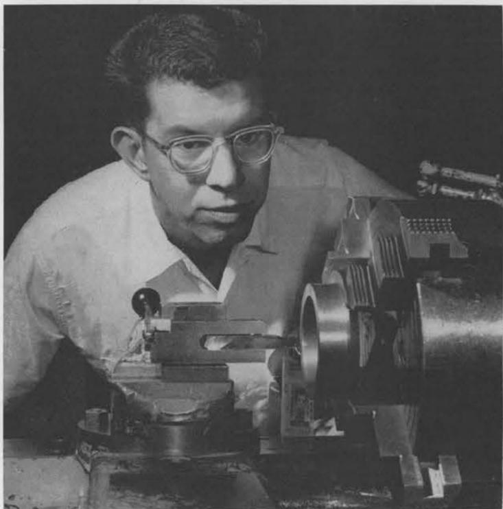
**WEARING SAFETY GLASSES** prevented possible eye injury when tool bit broke on lathe operated by Tony Saavedra (4251-1), above.
