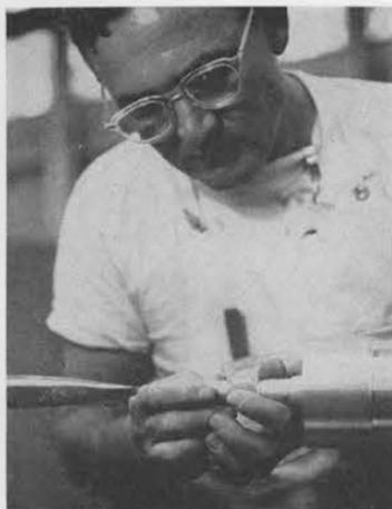
**SAFETY HAZARD** from sharp bit on lathe is shown by Earl G. Smith (4254-1). Picture below shows bit covered by rubber cube which is used to prevent scratches and punctures.
