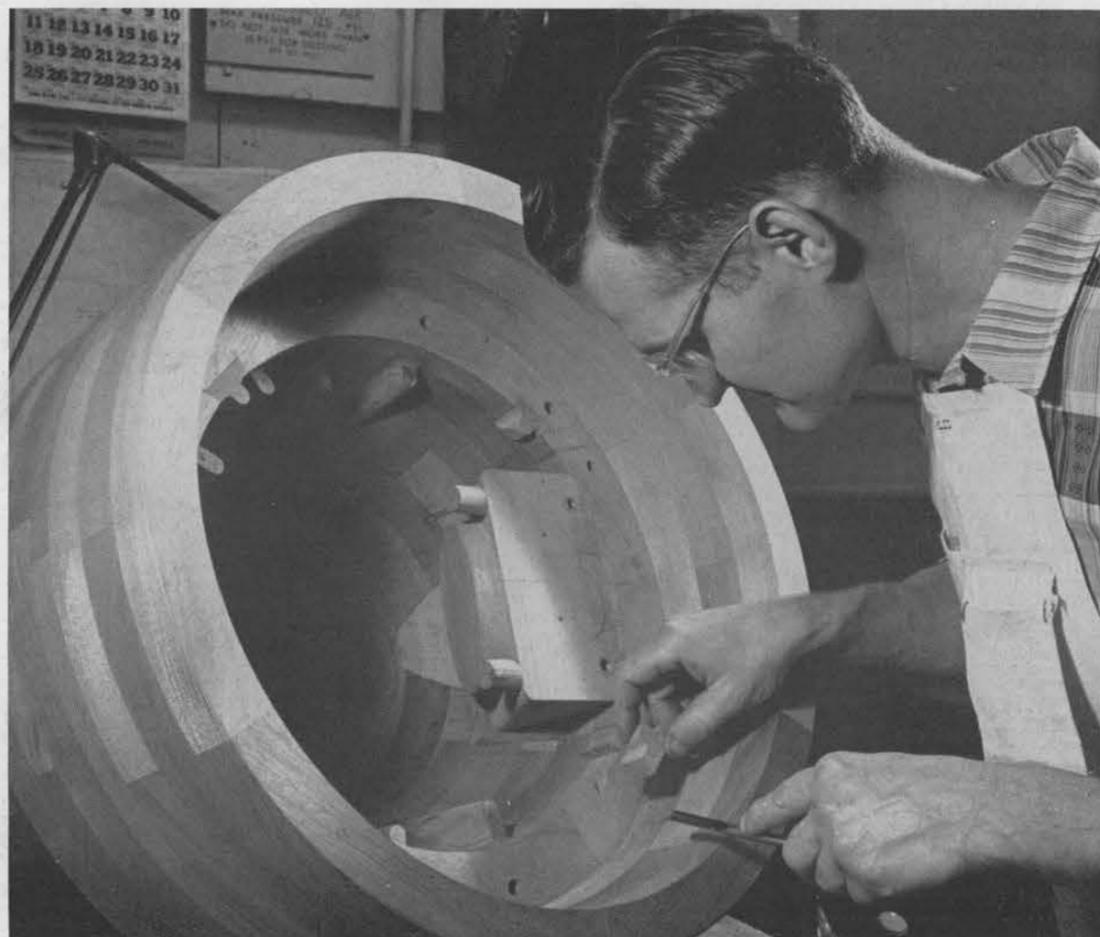
**NEARLY COMPLETED** tracking telescope mount pattern receives finishing touches from James Reed. Grain structure flowing in the circles is clearly visible in this photograph. Wood is Honduras mahogany, the hardest and most stable wood from which to machine and shape patterns.
