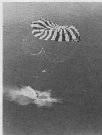
IMPACT of the full scale Project Mercury space capsule is shown during a test at Salton Sea Test Base. An inertia switch has fired an explosive charge disconnecting the 63 ft. parachute. Sandians are helping conduct the series of drop tests.
