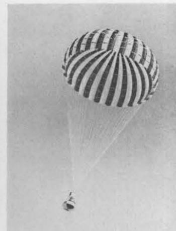
DESCENDING FROM 30,000 ft., the full scale Project Mercury Test Capsule travels at the rate of 30 ft. per second. Drop tests of the one-ton capsule at Salton Sea Test Base have been from a USAF C-130 transport and from a U. S. Marine Corps HR2S-1 helicopter.
