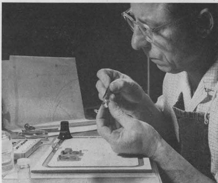
MINIATURE ODOMETER, used to measure lapsed distances, is being assembled by Ed Grymkowski. Large scale drawings, designed by engineering groups, have been used in tooling tiny parts.
