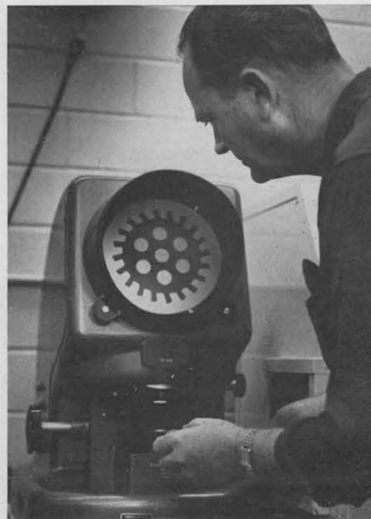
COMPARATOR is utilized by Vic Schaeffer in checking size and outline of tiny escapement wheel for a timing device against large scale drawing. Drawings are frequently of a 50 to one ratio.
