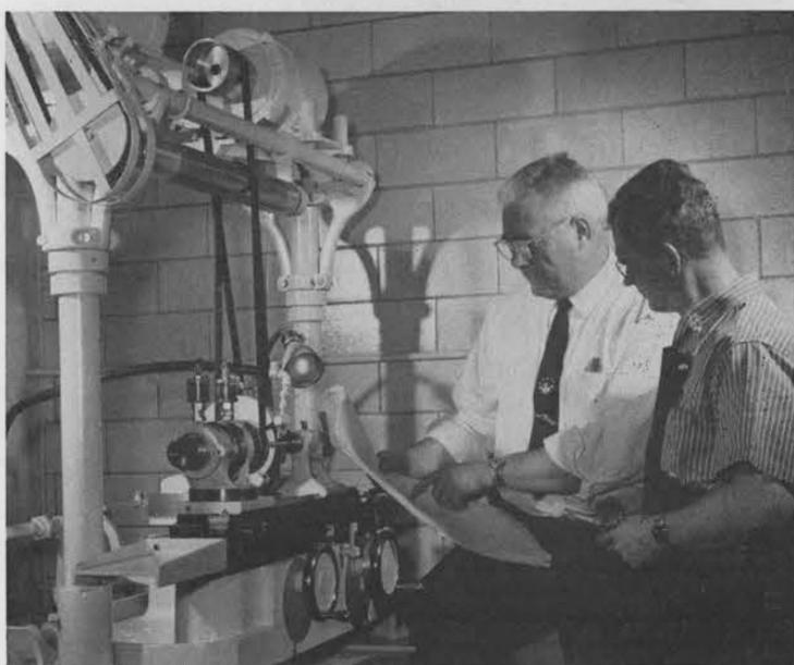
UNIVERSAL CYLINDER GRINDER has been operated by Rex Rozelle in forming this experimental mandrel for air bearing application studies. Supervisor C. C. Paschal checks dimensions.
