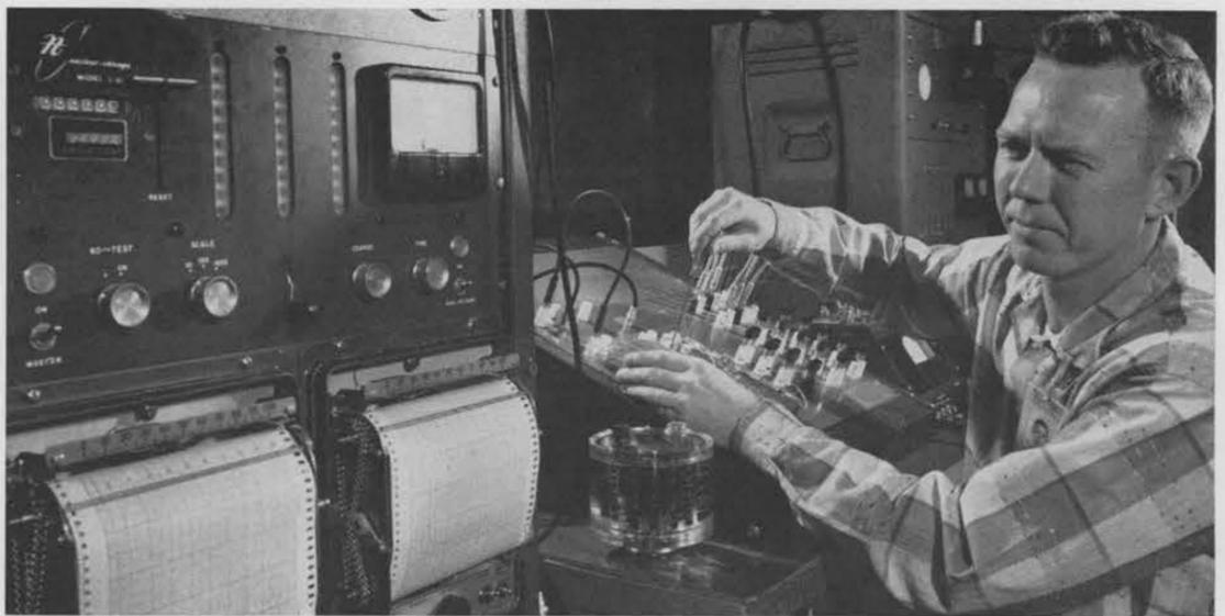
REJECTED COMPONENTS from the field are given "post mortem" analysis by Nathan Brown (5524-1) to determine exact cause of failure. Following precise electrical measurements the part will be further dissected to verify point of failure. Analysis equipment was designed by Nathan.
