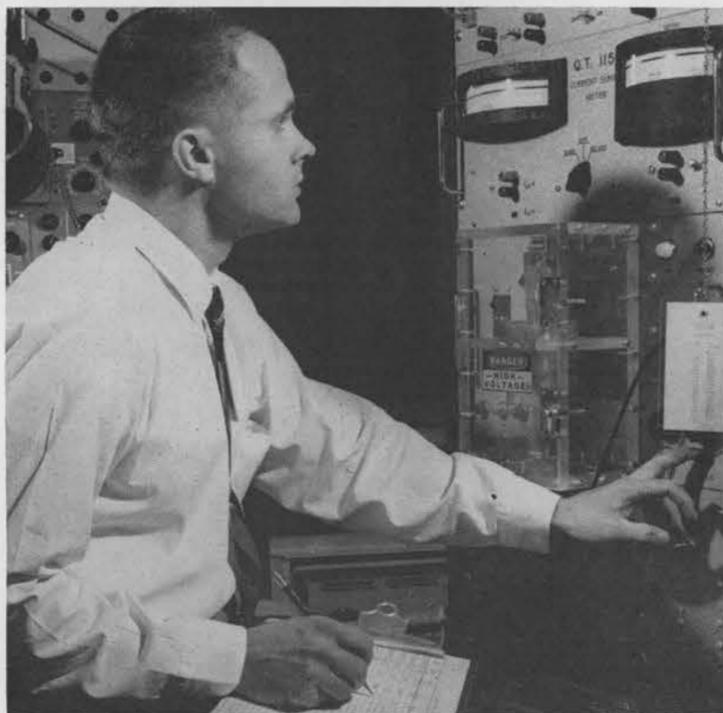
SUBJECTING CAPACITORS to rigorous leakage current and resistance tests is Art Cannon (5523-3) who determines their ability to meet stringent design specifications after periods of storage. Special test equipment like this QT-115 is designed by QA when no commercial equipment will make the necessary measurements.
