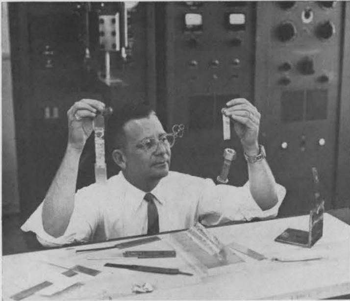
ULTRASONIC WELDING SAMPLES are displayed by L. E. Null (1621-2). At left he is holding a sample of thin aluminum foil welded to two pieces of glass. At right a thin wire weldment supports a heavy bolt. In the foreground are samples of dissimilar metals and materials that have been joined by ultrasonic process.
