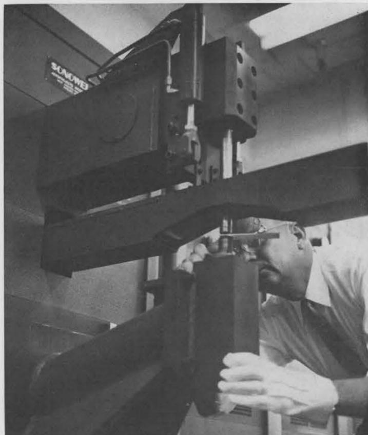
LARGE ULTRASONIC WELDING machine is operated here by L. E. Null. He is joining thin bars of aluminum and tungsten. Directly above the welding point is encased the steel "reed" that creates the ultrasonic vibration. Very little heat is generated.
