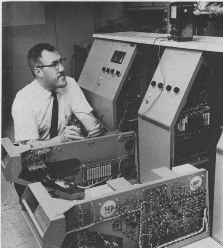
EASY ACCESS TO THE "innards" of Sandia's new high resolution mass spectrometer is shown in photograph above. Racks of components fold out for rapid checking such as J. W. Guthrie is performing. The instrument was the first commercially available one.
