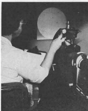
**NEUTRON TRACKS** are easily read on this microprojector which has magnified the film almost 800 times. Rita Hodgden, who is counting the tracks, uses this information in determining neutron exposure.
