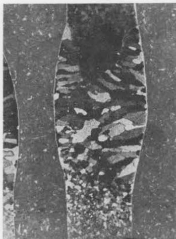
3. Photomicrograph as seen by Joe Darginis shows a cross section, greatly enlarged, of a weld of two dissimilar metals. Markings indicate grain growth of metal from the heat.
