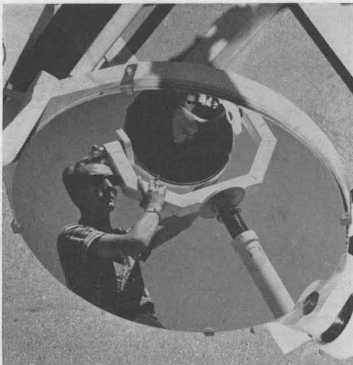
MIRROR SYSTEM shown in the photograph above reflects a constant beam of light through a tube in the wall of Bldg. 880 into the optical development laboratory of 7224-1. Large mirror rests on the ground and tracks the sun. Second mirror, being positioned by Bob Hughes, beams the light through the tube where Dan Fenstermacher is checking alignment with the optical bench inside.
