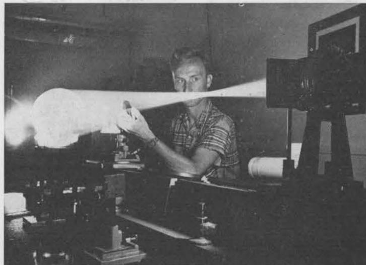
BOB HUGHES takes a light reading along the cone of sunlight reflected into the optical development lab through a hole in the side of Bldg. 880. By moving the test stand with the solar cell along the optical bench various intensities of light can be achieved.
