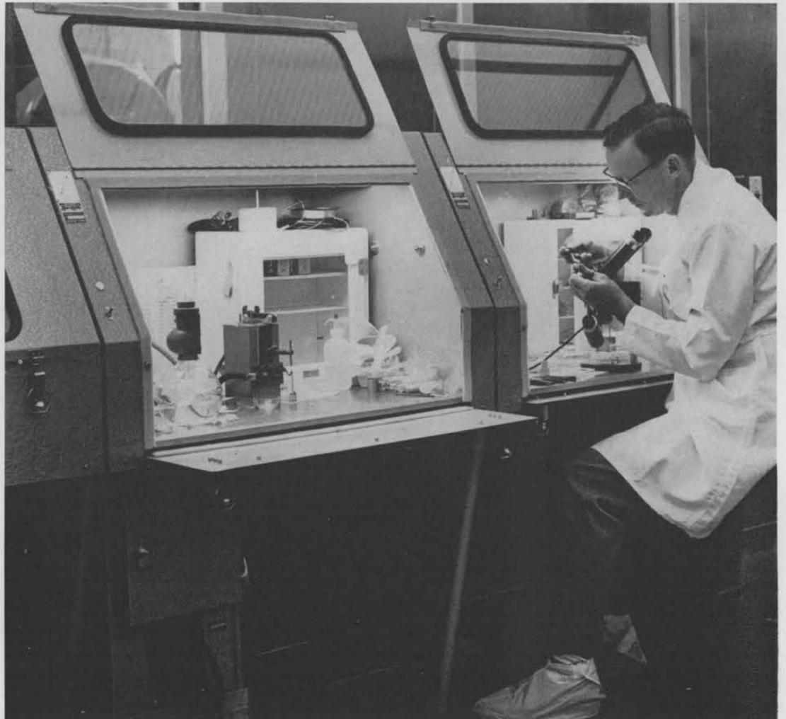
**MICROSCOPES**, welding and testing equipment are available at work benches inside Physical Electronics Laboratory clean room for final work on vacuum devices. Vernon Smith examines ceramic core.
